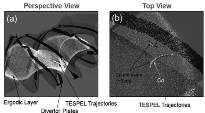
Fig. 2 (a) A perspective view of the three-dimensional trajectories of the TESPEL ablation clouds in the three different NBI heating cases, (b) an enlarged top view of the trajectories of the ablation clouds with showing the observed position of the LiI emission.
