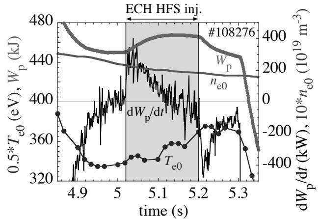
Fig. 1. Time evolutions of plasma stored energy  $W_p$  and its time derivative,  $0.5 \times T_{e0}$  and  $10 \times n_{e0}$  in the SDC discharge with HFS-ECH.
