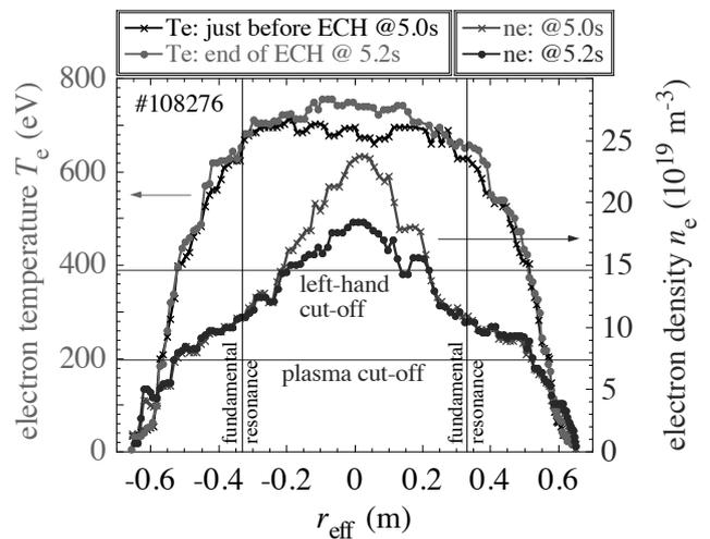
Fig. 2 Profiles of  $T_e$  and  $n_e$  at just before and at the end of ECH pulse in the SDC discharge with HFS-ECH.
