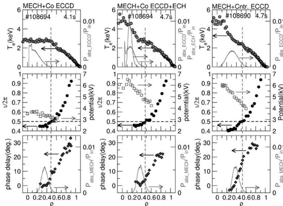
Fig. 1. (From the top) Profiles of the electron temperature ( $T_e$ ) and power absorption of ECCD. Profiles of the rotational transform ( $\nu/2\pi$ ) and plasma potential. Profiles of the phase delay of 25Hz modulated heat pulse and power absorption of MECH.
