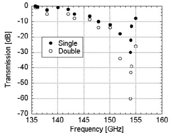
Fig. 3. Transmission property as a function of frequency.
