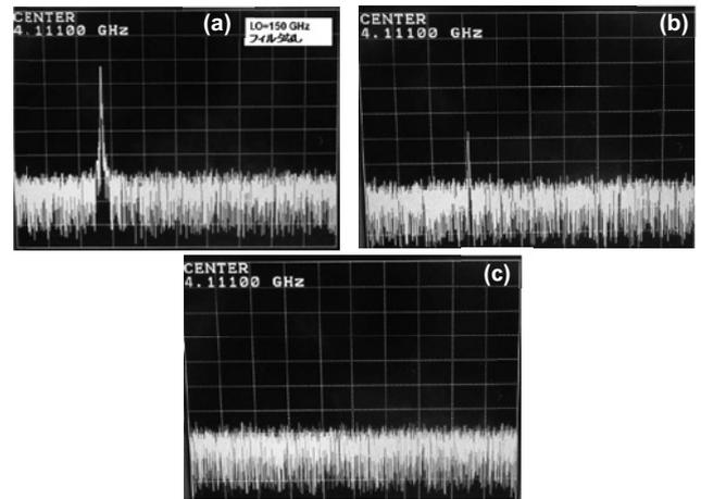
Fig. 2. Measured spectra of sub-harmonic mixer output with (a) no filter, (b) single-layer filter, (c) double-layer filter. center frequency 4.111 GHz, vertical scale 10 dB/div, horizontal scale 20 MHz/div.
