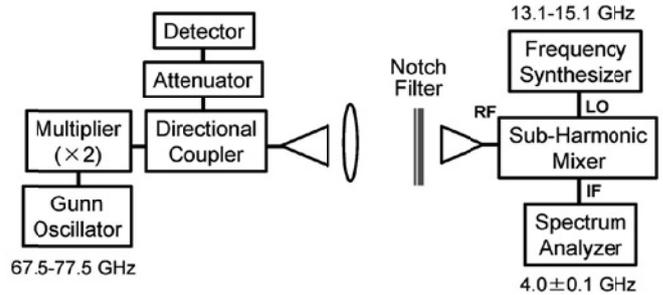
Fig. 1. Schematic of the FSS notch filter testing setup.
