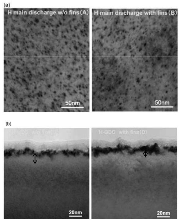
Fig. 2: (a) Blight-field images of specimens at the bottom of the cylinder (A) w/o and (B) with fins exposed to hydrogen main discharges. (b) Thickness of the impurity deposition (shown with arrows) (C) w/o and (D) with fins exposed to hydrogen during glow discharges.
