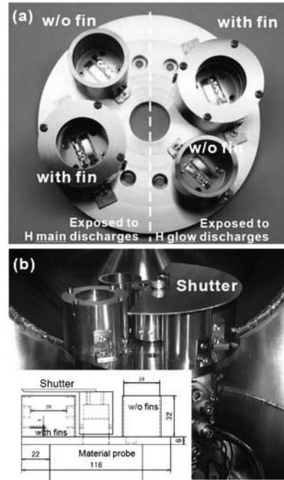
Fig. 1: (a) two sets of cylinders with and without fins. (b) Cylinders put on the material probe
