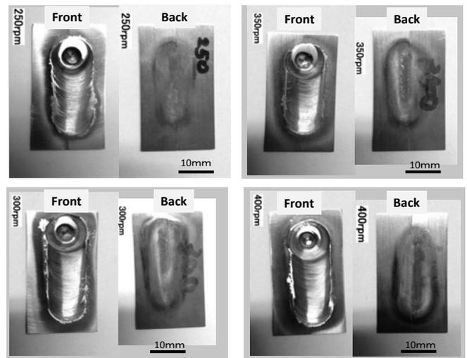
Fig. 2 Top and bottom surfaces of ODS joint by FSW.
