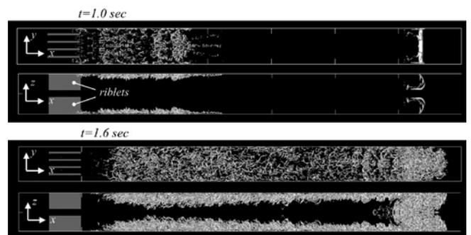
Fig. 2: Vortical structure in the case of vertical channel with riblets.
