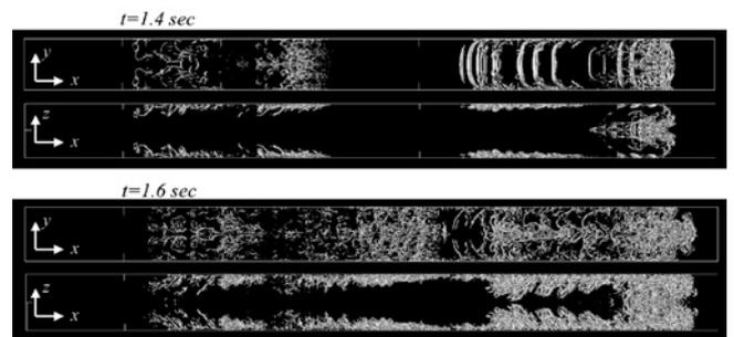
Fig. 1: Vortical structure in the case of vertical channel without riblet.
