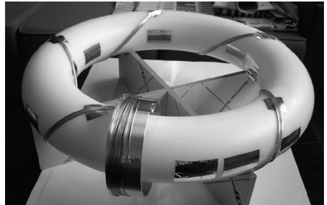
Fig. 2. Model of helical winding core on which a coil case is wound by five turns. A stainless wire corresponds to CIC conductors.
