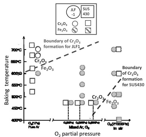
Fig. 2 Influence of baking temperature and O<sub>2</sub> partial pressure on the oxidized composition.
