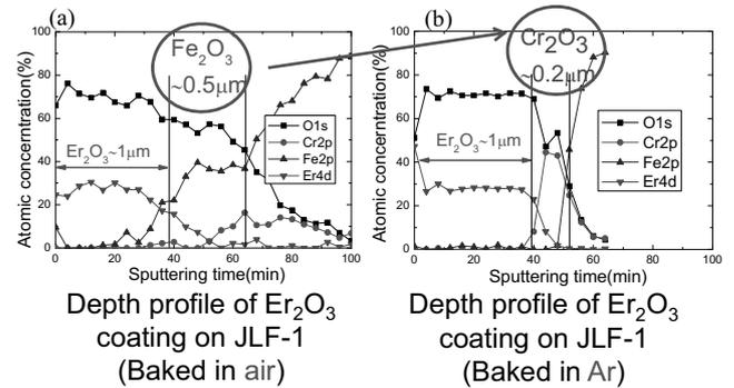
Fig. 1 Element depth profiles of Er<sub>2</sub>O<sub>3</sub>-coated JLF-1 plates. (a) Baked in air. (b) Baked in Ar (O<sub>2</sub>: ~1 ppm as impurity).
