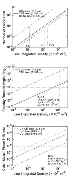
Fig. 1: Phase shifts of dispersion interferometer (a), the Faraday rotation angles (b) and the Cotton-Mouton phase shift (c) on a helical DEMO reactor, which is four times larger than LHD.
