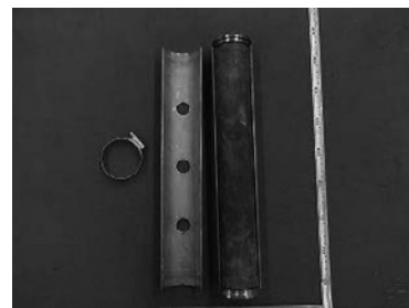
Fig. 4 Jigs for the preparation of tubular cells
