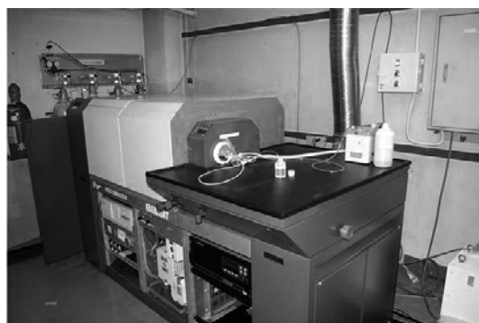
Fig. 1 Double focusing sector field type ICP-MS instrument (Finnigan MAT ELEMENT)
