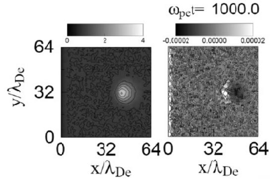
Fig. 2: Electron density distribution (the left panel) and distribution of the  $y$  component of electric current density (the right panel) in the  $x$ - $y$  plane at  $z = L_z/2$  at  $\omega_{pe}t = 1000$ .
