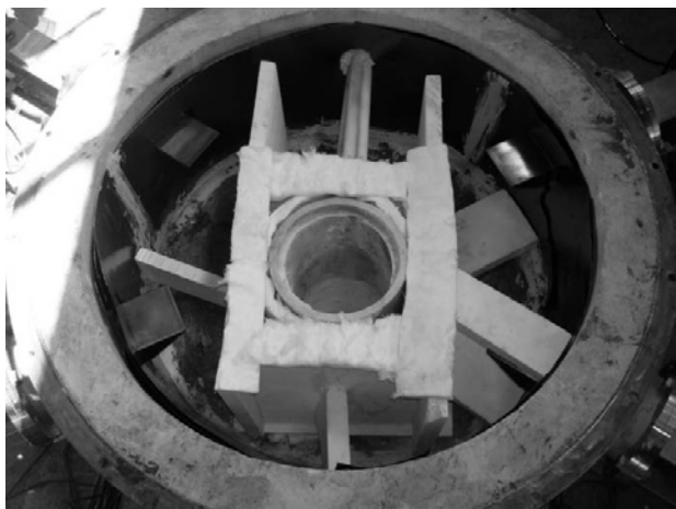
Figure 1 Load chamber for 120kW at 2.45 GHz and reaction furnace
