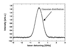
Fig.2. LIF spectrum for argon neutral particles.
