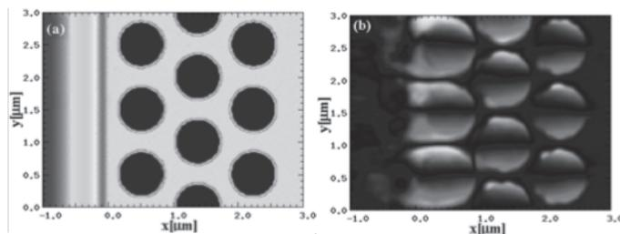
Fig.2. Punched out target. (a) electron density profile and (b) quasi-stationary transverse magnetic field profile.
