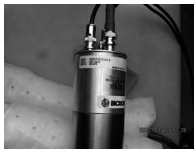
Fig.2 Neutron detector installed on EAST for collaboration on high-energy particle and MHD studies
