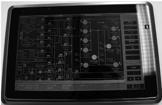
Fig. 22. Tablet PC for remote monitoring.
