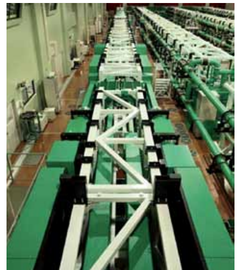
Fig. 2 Amplifier chain of the LFEX laser beams.
