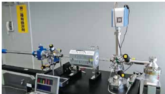
Fig. 2 Thermal desorption device installed in Hydrogen Isotope Research Center, Organization for Promotion of Research, University of Toyama for measurements of H, D and T.
