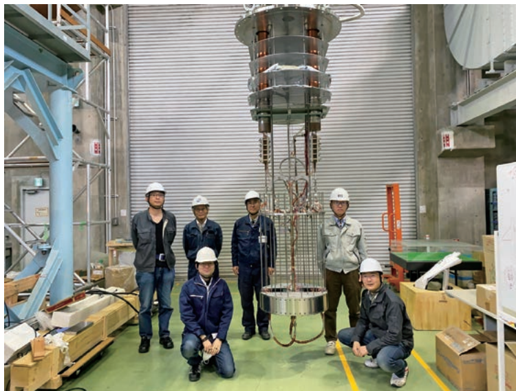
Fig. 9 A 6-m-long coiled HTS-STARS conductor sample and the research team.
