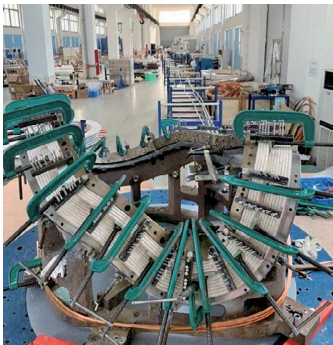
Fig. 1 A modular coil in the winding process
