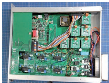
Fig. 3 DC offset voltage canceller.
