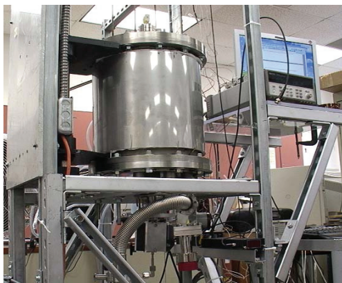
SiC/pebble bed thermomechanics test set-up with Keyence laser position system for displacement measurement
