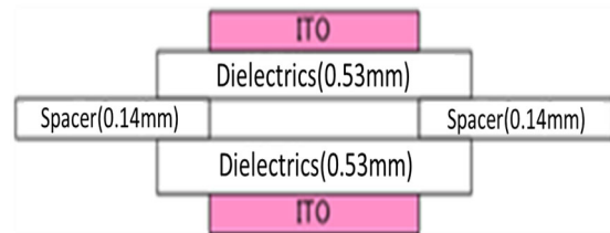
Fig. 1. Schematic of a microgap discharge cell
