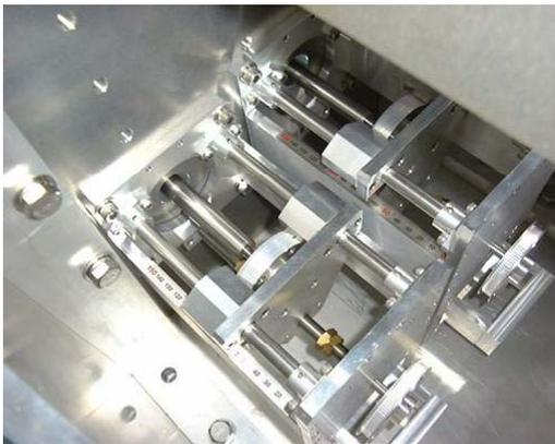
Fig.4 Sliding bearing
