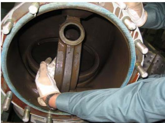
Fig. 8 Inside of damaged valve
