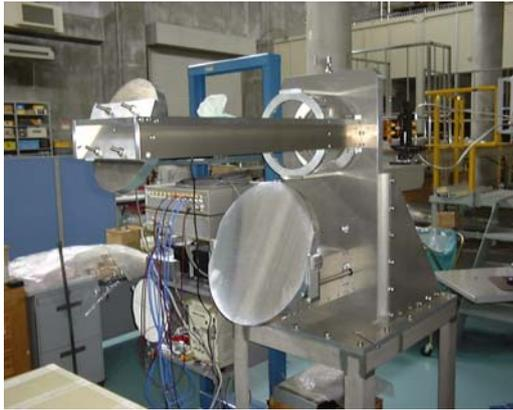
Fig.3 Microwave Imaging Reflectometer (MIR)
