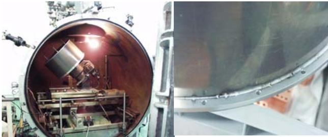
Fig.4 EBW of aluminum alloy.
