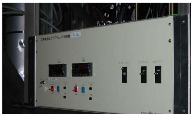
Fig. 20 Control box of the liquid stub tuner
