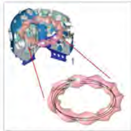
IMAGE: LH2 HIGH-ENERGY PARTICLES CIRCULATE INSIDE A PLASMA THAT IS SHAPED LIKE A TWISTED DOUGHNUT, AND THEY CAUSE PLASMA OSCILLATIONS. IN PARTICULAR, WHEN THE PERIOD OF THE CIRCULATION AND THAT OF... view more >
