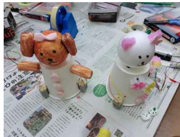
Completed robots. The vibration by the motors drives them forward.
