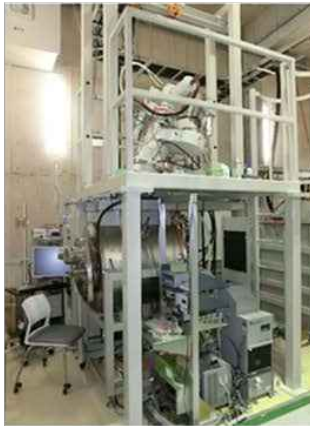
High Heat Flux Test (ACT2)
