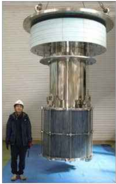
13 T, \phi 700 mm Solenoid Coil
