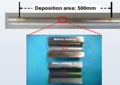
Er<sub>2</sub>O<sub>3</sub> coating on the tube interior
