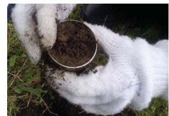
Passive type sampler (atmospheric water vapor)
