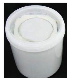
Passive type sampler (atmospheric water vapor)
