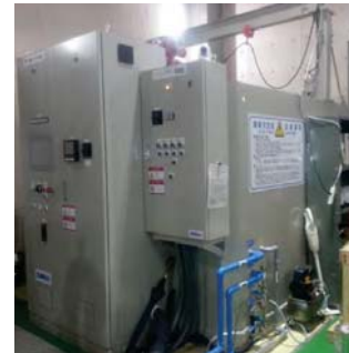
Hot Isostatic Press (HIP) facility
