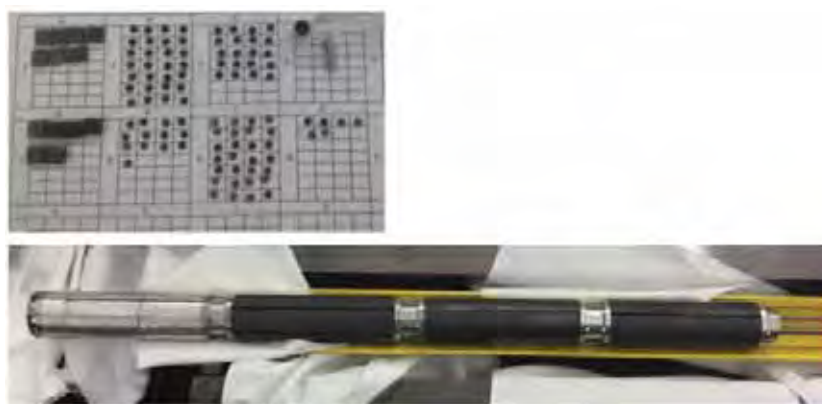
Figure 4.3.1-1 W alloy samples fabricated by NIFS collaborations and HFIR irradiation capsules.
