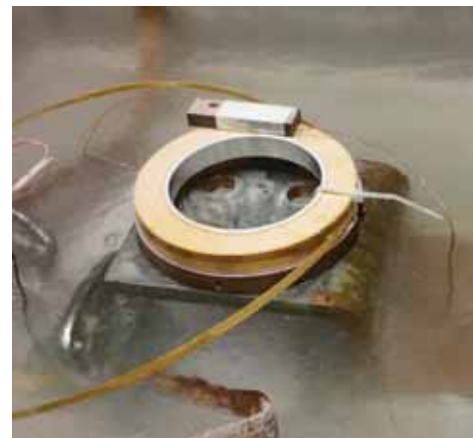
Figure 4.3.5.3-2 Photograph of the cool-down (immersed in liquid nitrogen) and excitation test of a trial HTS coil at NIFS.
