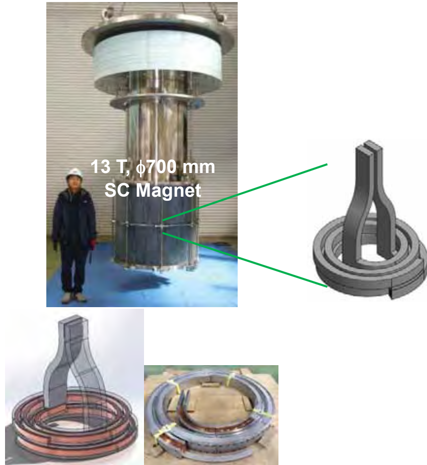
Figure 3.3.1.3-15 Schematic illustration of a HTS STARS conductor to be tested in the new superconductor testing facility at NIFS equipped with a 13-T magnetic field and 700-mm bore solenoid coil. The rated current is 30 kA at temperature 20 K.
