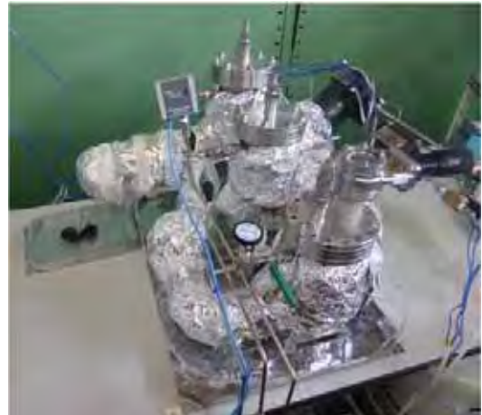
Figure 3.3.4.2-8 Gas driving liquid loop operating with FLiNaK at around 800 K.
