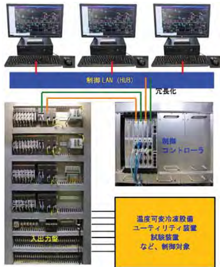
Figure 3.3.2.1-2 Control system configuration.
