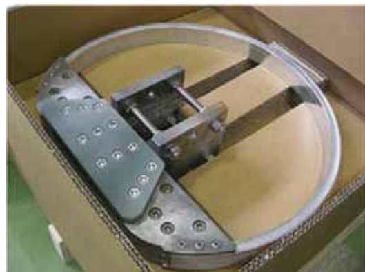
Figure 3.3.1.2-9 Photograph of 1-turn winding sample for a demonstration test.
