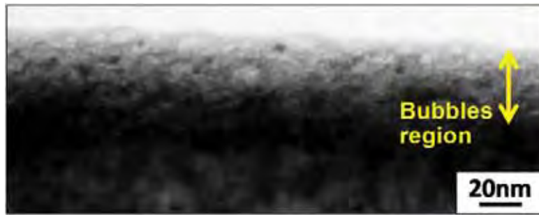
Figure 3.3.5.3-4 Cross-sectional TEM image of VPS-W/IG divertor tile after used to LHD plasma experiment [3.5.3.9].
