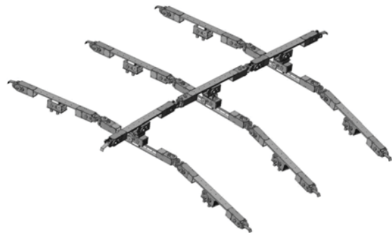
Figure 3.2.7.5-5 Variable structure with a combination of joint-type robots.
