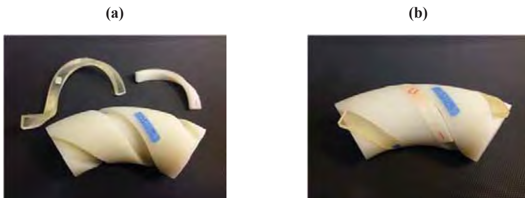
Figure 3.2.4.4-6 Confirmation of HTS joint-winding by 3-D printing models.
