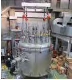
Performance tests of the JT-60SA CS model and module coils
