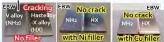
EBW of V alloy and hastelloy with or w/o Ni or Cu filler Reinforcement of the ferritic steel material by joining with ODS
