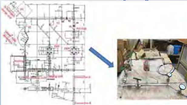
Hydrogen monitoring and trapping with Y-Nb for flowing Li
