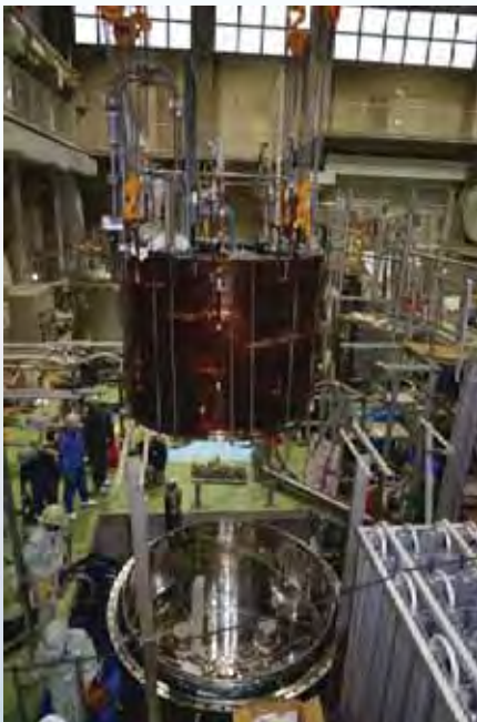
JT-60SA Central Solenoid (one module) was tested at NIFS SCM Lab.
