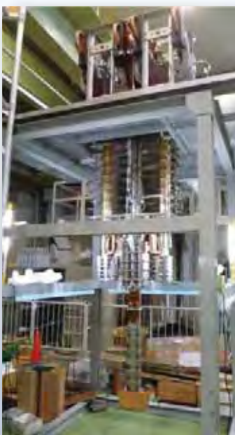
Performance test of a ITER-TF joint sample at NIFS
