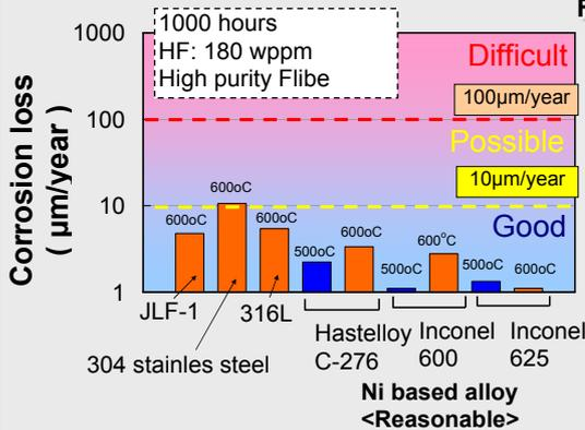
✓Corrosion tests in high purity Flibe were performed. Corrosion rate and mechanism in static condition was made clear.
