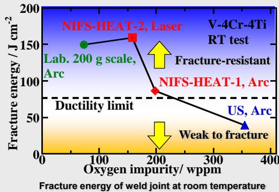
✓ High purity large scale V-4Cr-4Ti alloy ingots, NIFS-HEAT-1 and -2, were fabricated and distributed to world research institute.
