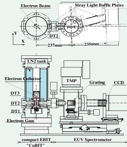
Fig.1 Cross sectional view of compact EBIT and EUV spectrometer
