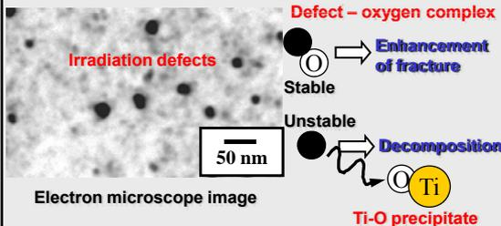
✓ It is believed that appropriate post-weld heat treatment (PWHT) forms Ti-O precipitates, and promotes decomposition of the defects
