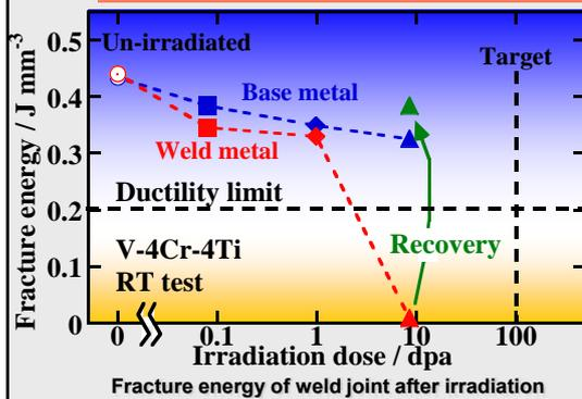
✓ Weld metal maintained high fracture energy until 1 dpa, while it degraded at 8.5 dpa.
