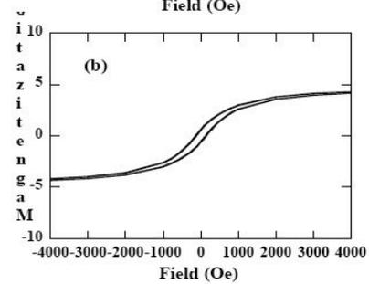
Fig.4 Magnetization curve of samples heated by magnetic field at (a) 1000 degree Celsius and (b) 1200 degree Celsius.
