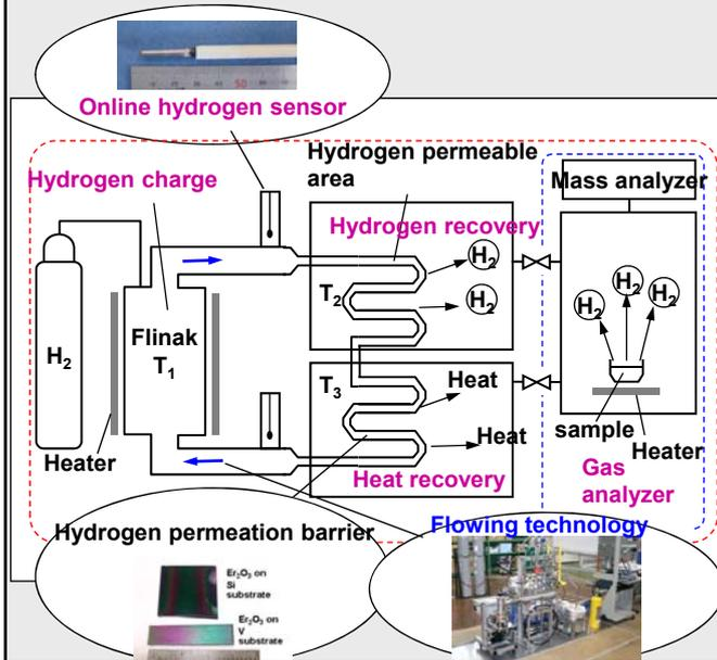
System integration for the feasibility studies on compatibility of **hydrogen recovery and heat exchange** in the flowing system is planned with the use of **Flinak** towards the Demo reactor.
