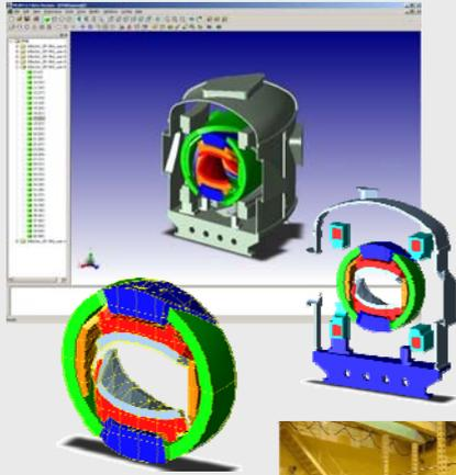
CAD geometry imported into conversion system MCAM, developed by ASIPP, CHINA
