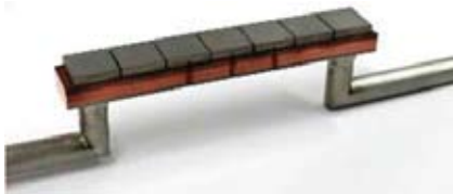
Prototype divertor heat removal component of W/ODS-Cu, fabricated by AMSB
