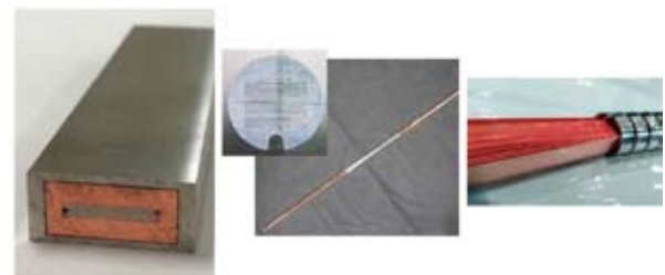
Large-current HTS conductors for application in next-generation fusion experimental devices (left: STARS, middle: FAIR, right: WISE)
