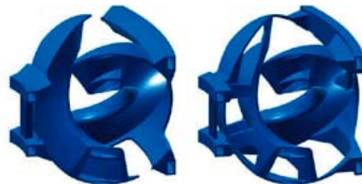
Conventional design (left) and a topology-optimized one (right) for the coil supporting structure (a part of a doughnut is shown for both).
