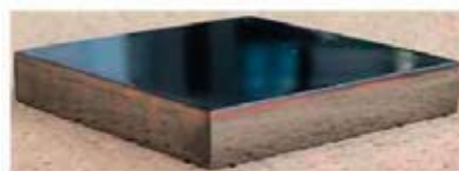
Joint sample of tungsten sheet and stainless steel, fabricated by AMSB
