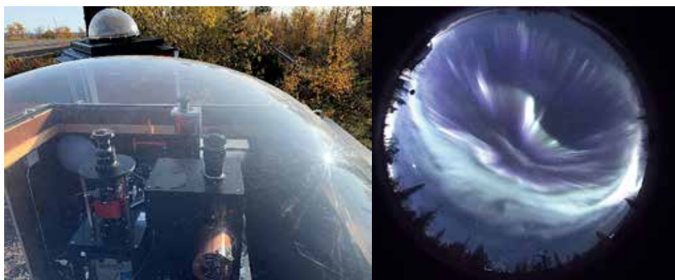
Fig.2 Aurora Spectroscopy Measurement System (left) and aurora image taken by all-sky camera (right).
