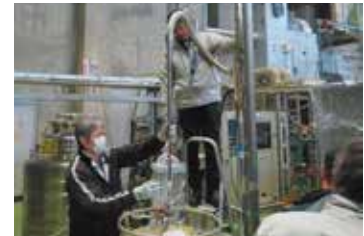
Liquid helium transfer operation
