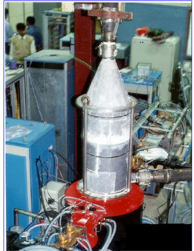
KLYSTRON 2103D WITH DIRECTIONAL COUPLER
