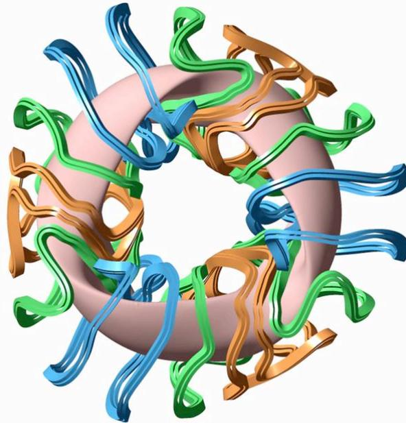
Coils wound on forms to create a robust structural shell minimizes deflections
