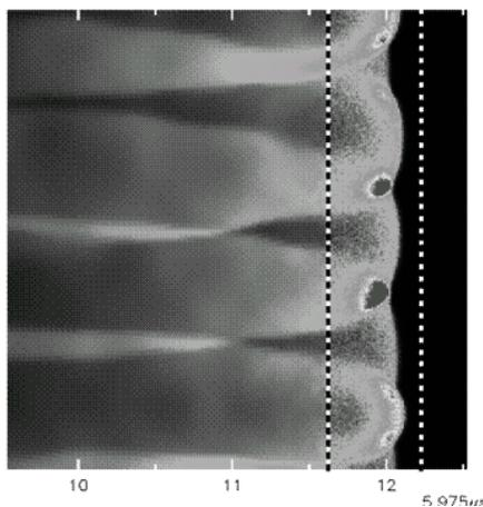
Fig. 2 The pressure distribution of the detonation simulation. The particle-based domain, which corresponds to the region bounded by dotted lines, tracks the detonation front.
