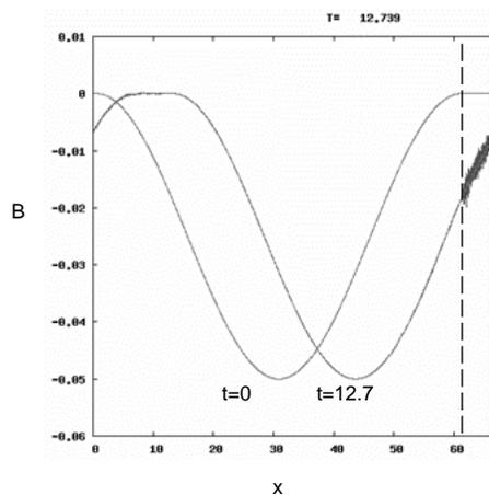
Fig. 3 Magnetic field distribution in the test simulation for Alfvén wave using the PIC-MHD interlocked model. The region between two dotted line corresponds to the part where PIC model is embedded.
