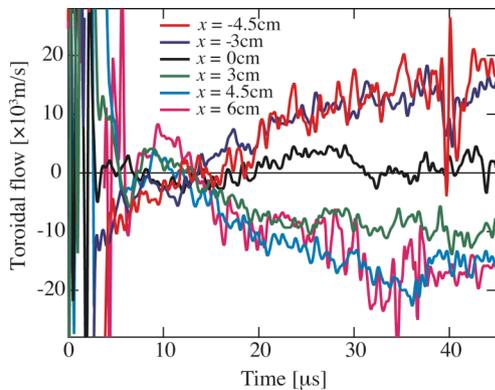
Fig.2 Time evolution of toroidal flow velocity measured by the IDS measurement.
