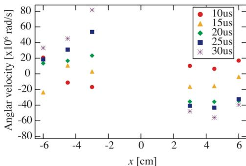
Fig. 3 Time evolution of radial profile of toroidal angular velocity.
