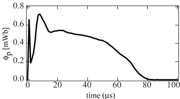
Fig. 5 Time evolution of the poloidal flux estimated under the assumption of rigid rotor profile model.
