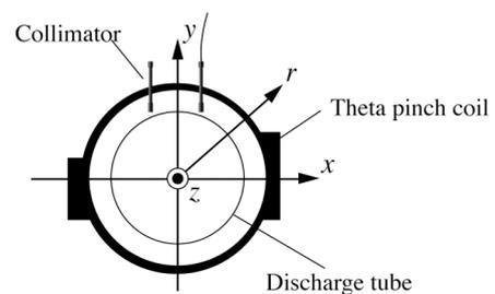
Fig.1 Toroidal section of NUCTE-III device and arrangement of collimators for IDS.
