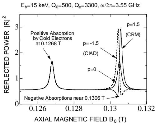
Fig. 3 Curves of absorption expected for CRM (solid curve) and CIAD (dashed curve).
