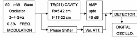
Fig. 4 Constructed microwave interferometer circuits including fabricated TE<sub>011</sub> mode cylindrical two-port cavity with resonant frequency near 3.45 GHz.
