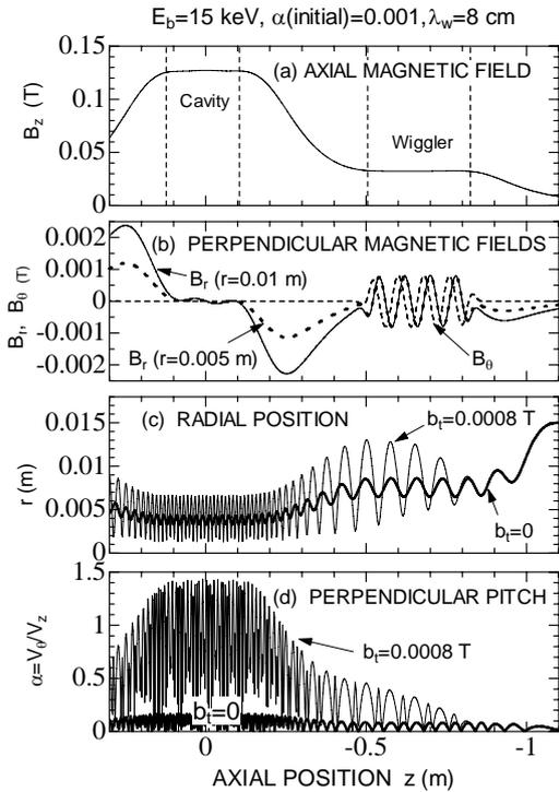
Fig. 2 Electron beam properties obtained by trajectory tracking. Helical field  $b_t$  enhances significantly perpendicular pitch  $\alpha = V_\theta / V_z$ .
