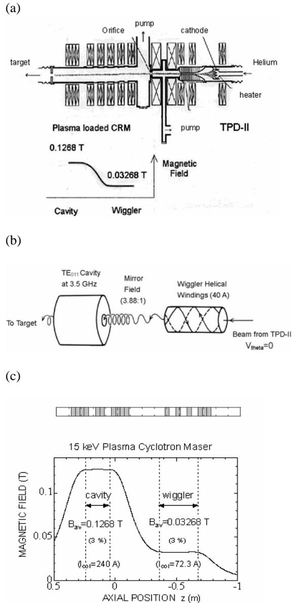
Fig. 1 Plasma-loaded CRM installed inside the TPD-II Machine, NIFS, Japan. (a) Total view. (b) Principle of plasma-loaded CRM. (c) Distribution of axial magnetic field in the wiggler and the cavity. Bar code shows the location of 16 coils.
