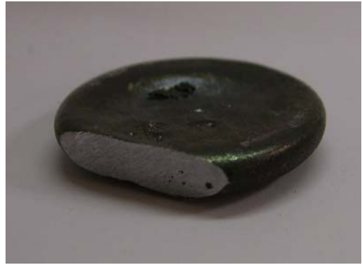
Fig.3 Pig iron from the 30GHz mm-waves process.
