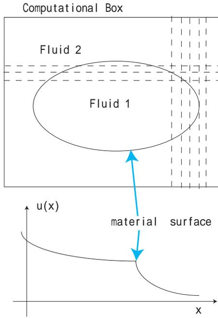
Fig. 1 A schematic view of two fluids separated by a material surface.
