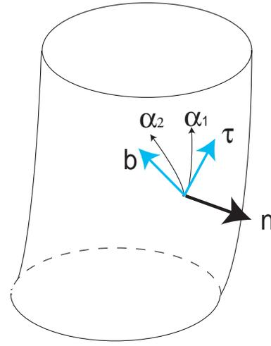
Fig. 2 Coordinate lines  $\alpha^1, \alpha^2$  which cover the material surface and the tangential, normal and binormal unit vectors.
