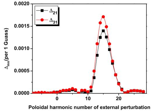
Fig. 2 (a) The typical poloidal harmonic coupling spectrum between the Fourier components of the external error field on the plasma boundary  $(\delta\mathbf{B}^x \cdot \mathbf{n}_b)_{mn}$  and the total resonant field, which is here measured by  $\Delta_{21}$  and  $\Delta_{31}$ .
