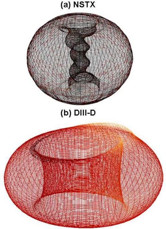
Fig. 1 The deformed plasma boundary of typical (a) NSTX (b) DIII-D tokamak plasmas due to each intrinsic error field. The scale is arbitrary.
