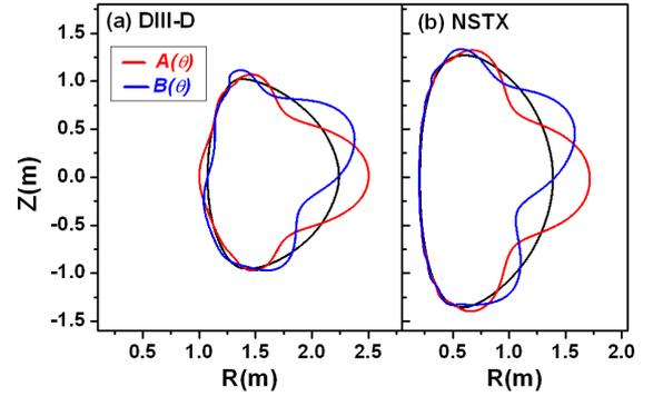
Fig. 3 The most important external field driving the total resonant field on rational surfaces, in the (a) DIII-D and (b) NSTX. The three dimensional distribution can be constructed by  $\delta\mathbf{B}^x \cdot \mathbf{n}_b = A(\theta)\cos(\phi) + B(\theta)\sin(\phi)$  relative to the plasma boundary (black line).
