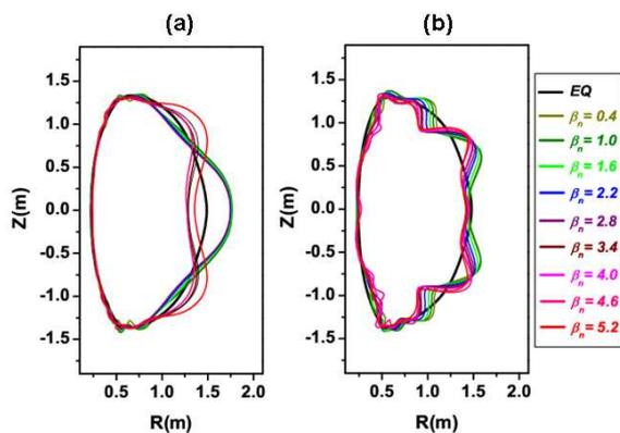
Fig. 4 (a) The most important  $n = 1$  external field and (b) the  $n = 1$  external field driving only  $l = 1/2$  as a function of  $\beta_n$  in NSTX. The external fields are represented relatively to the plasma boundary as in Fig. 3.
