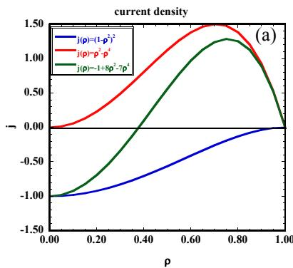
Fig. 8 (a) Toroidal current profile and (b) Radial profile of rotational transform deduced from VMEC calculation with the effect of toroidal current and plasma pressure.
