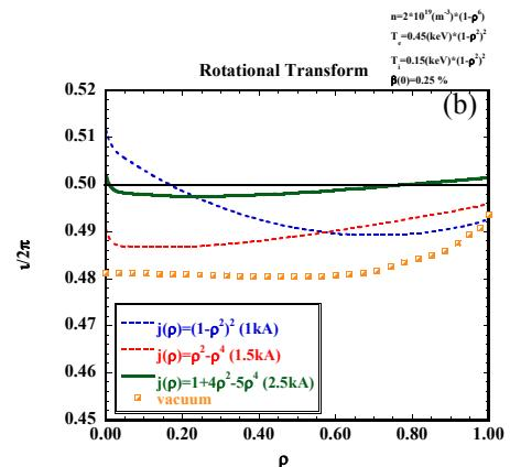
Fig. 5 (a) Toroidal current profile and (b) radial profile of rotational transform deduced from VMEC calculation with the effect of toroidal current and plasma pressure.
