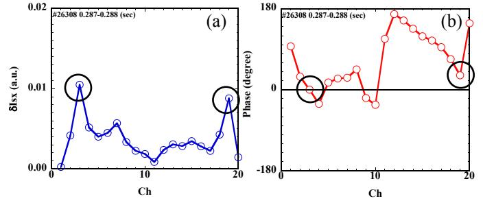
Fig. 7 Radial profile of (a) SX fluctuation amplitude and (b) phase difference among SX channels.
