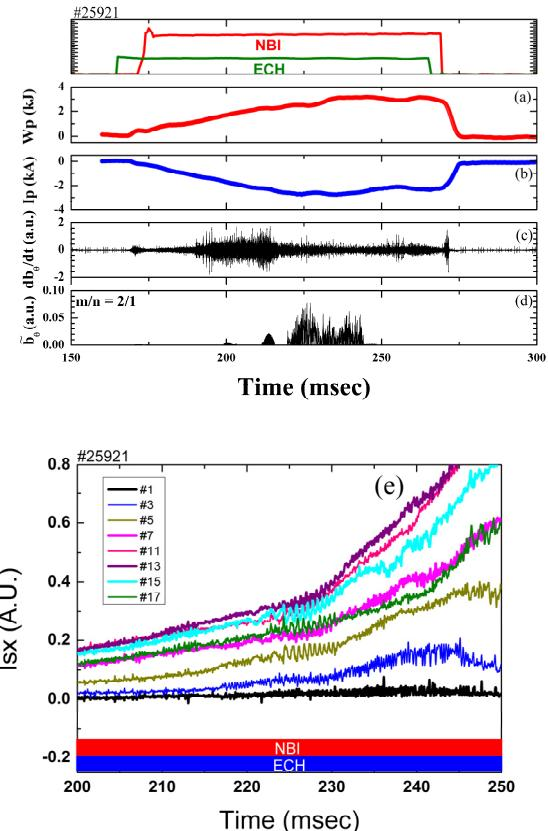
Fig. 3 Time evolution of an ECH + co- NBI plasma. The (a) stored energy, (b) toroidal current, (c) magnetic fluctuation, amplitude of (d)  $m/n = 2/1$  and (e) extended view from 200 msec to 250 msec of SX signals.
