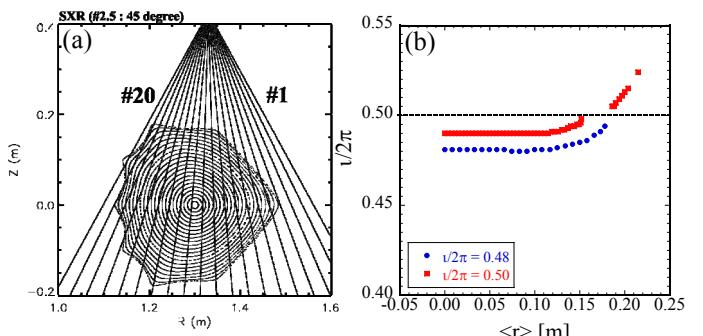
Fig. 1 (a) Magnetic flux surface and 20 lines of sight in SX array are shown. Radial profiles of rotational transform in vacuum condition are shown in (b).
