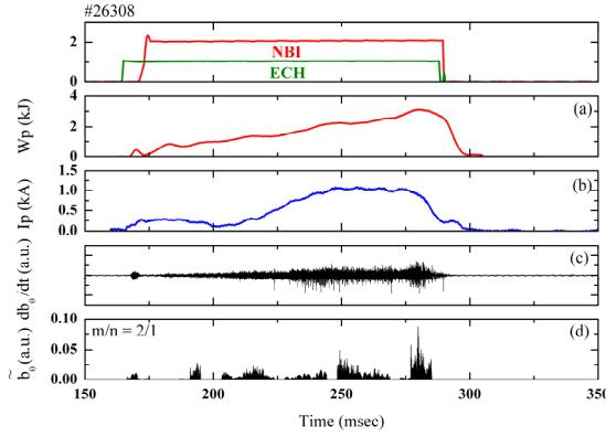
Fig. 6 Time evolution of an ECH + counter-NBI plasma. The (a) stored energy, (b) toroidal current, (c) magnetic fluctuation and amplitude of (d)  $m/n = 2/1$ .
