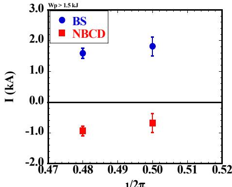
Fig. 2 Estimated bootstrap current and NB current.
