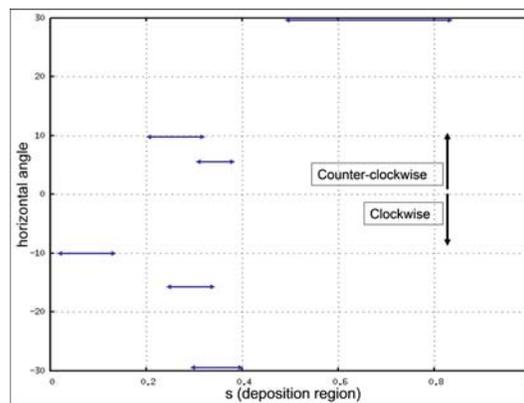
Fig. 7 Table indicating the power deposition region with respect to horizontal launching angle for the Heliotron-J XB conversion experiment.
