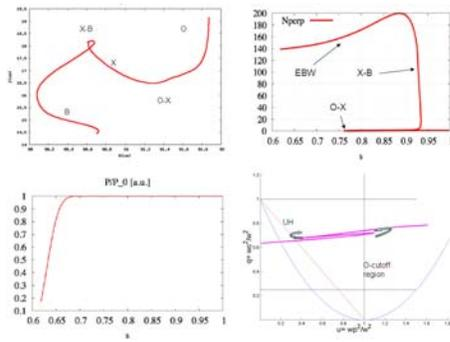
Fig. 2 Numerical results of the OXB simulation for CHS shot 129213. Ray path in R-Z coordinates (top left),  $N_{\perp}$  (top right), normalised power deposition profile (bottom left) and CMA diagram of the ray evolution (bottom right) profile
