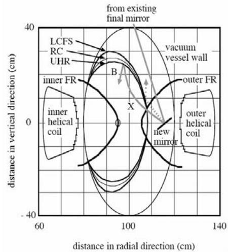
Fig. 3 CHS XB experiment launching scheme. The mirror is aimed at the region where the fundamental harmonic on the last flux surface.
