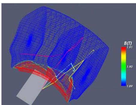
Fig. 6 Sample rays experiencing XB conversion when launched from the inner side of the torus simulating evolution after reflection in the inner wall. They represent reflections towards the clockwise, counter-clockwise and downwards directions. The scale of the magnetic field strength has been chosen to highlight the fundamental resonance region.
