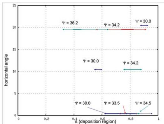
Fig. 5 Table indicating the power deposition region with respect to horizontal launching angle. The vertical angle of each simulation is also indicated. The thin lines represent partial X-mode absorption and the thick lines indicated Bernstein wave absorption.
