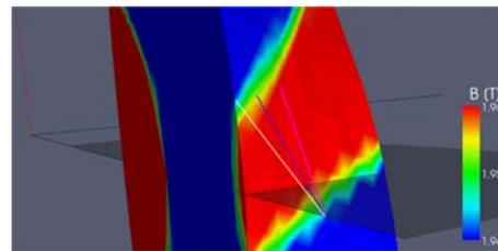
Fig. 4 CHS launching position and angles for the XB heating experiment. The scale of the magnetic field strength has been reduced in order to highlight the fundamental resonance stripe on the las magnetic surface.
