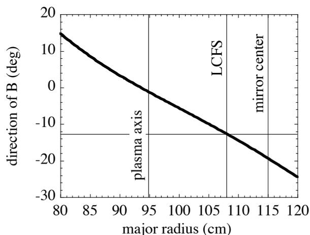
Fig. 4 Variation of the magnetic field direction along a beam path perpendicular to the flux surfaces.
