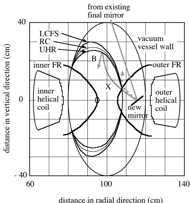
Fig. 1 Experimental configuration for slow X-B experiment.
