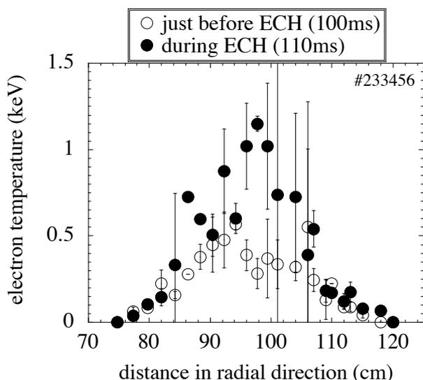
Fig. 3 Electron temperature profiles just before EC-wave injection and during injection measured using Thomson scattering measurement.
