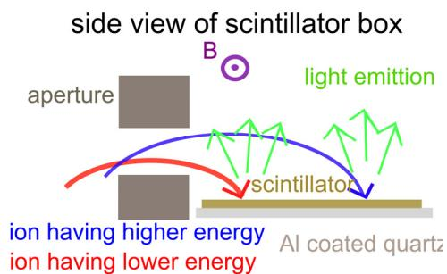
Fig.5 The side view of scintillator box. Lost energetic ions pass through apertures, and then hit a scintillator surface. Strike point gives information of both gyroradius and pitch angle of the lost ion.
