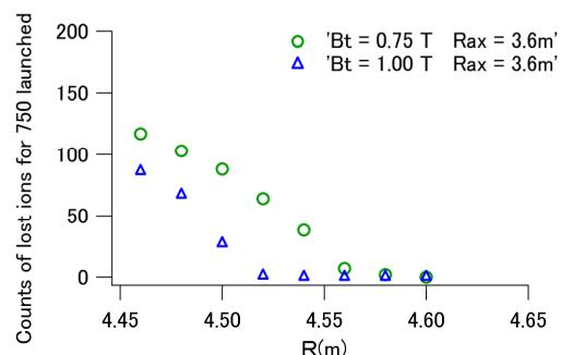
Fig.3 Counts of energetic ions that are lost from the plasma core region and reach to the LIP, where 750 particles are launched from the probe, having various energies and pitch angles. In the configuration of  $R_{ax} = 3.6\text{m}$ . The results at  $B_t = 0.75\text{T}$  and  $1\text{T}$  are shown by circles and triangles, respectively.
