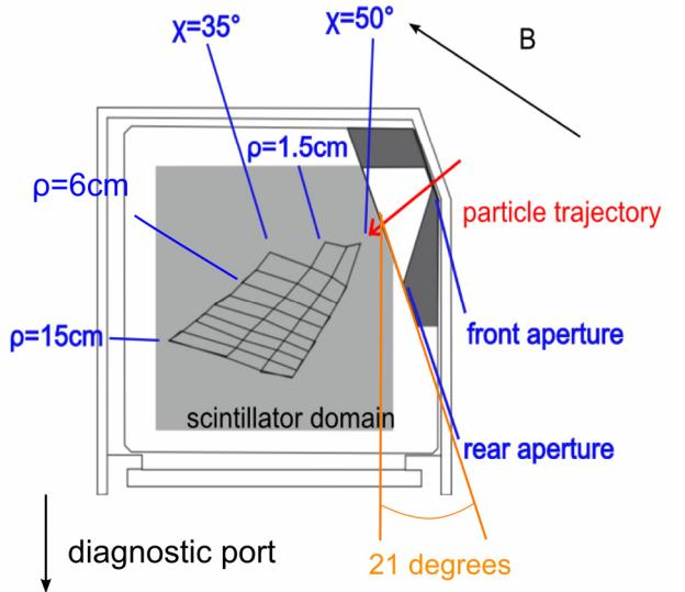
Fig.6 Schematic view of the probe head and expected arrival area of energetic ion. Expected hit point area of lost ions having the range of 1.5 to 15 cm for gyroradius and 35 to 50 degrees. The normal vector of the aperture is 113 degrees with respect to the local magnetic field direction. The size of a front aperture is 3 mm (width)  $\times$  1 mm (height) and the size of a rear aperture is 24 mm (width)  $\times$  1 mm (height). The distance between two apertures is 10 mm.
