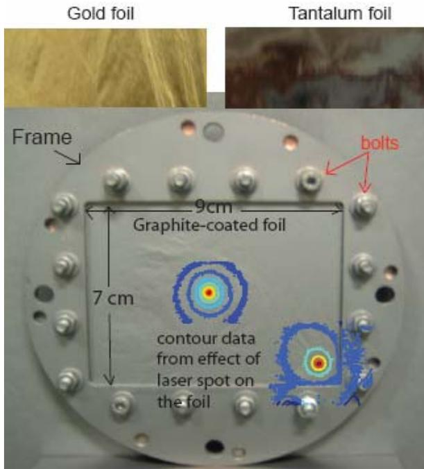
Fig.1 The single graphite-coated (one for Ta and one for Au separately) foil that is supported by a copper frame and temperature contour images from the laser spot after focusing on the foil (center and edge).
