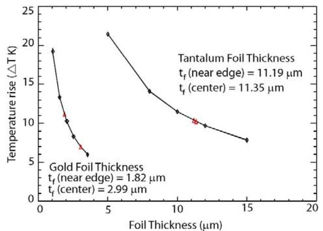
Fig.2 The appropriate value of the product of the  $kt_f$  of the (Au and Ta) foil from the experimental value of the  $\Delta T$  is found from fitting a second order polynomial to the  $kt_f$  and the  $\Delta T$  data from the FEM.
