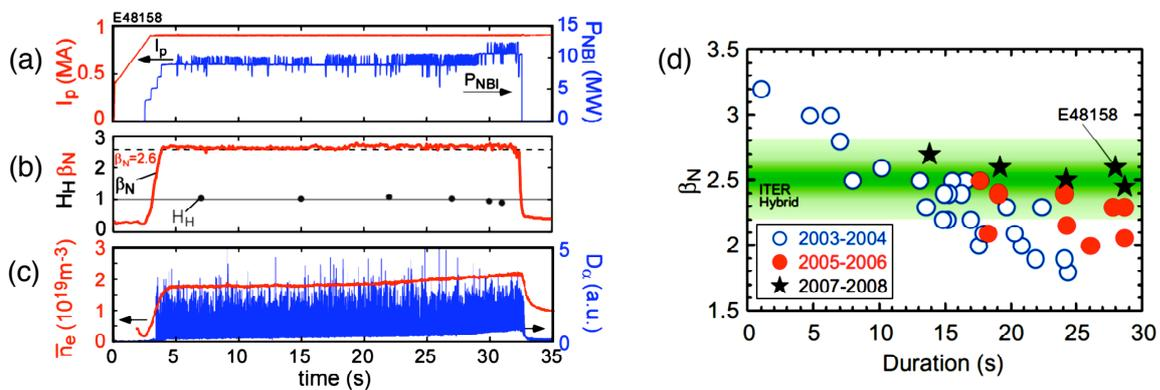
Fig. 1: Typical discharge of long-duration, high-beta plasma. (a) Plasma current and neutral beam power, (b) normalized beta and confinement enhancement factor and (c) line-averaged electron density and  $D_\alpha$  intensity. (d) Progress in  $\beta_N$  and sustained period.
