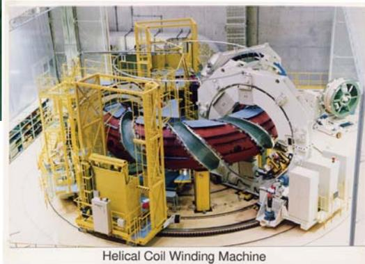
Helical Coil Winding Machine
